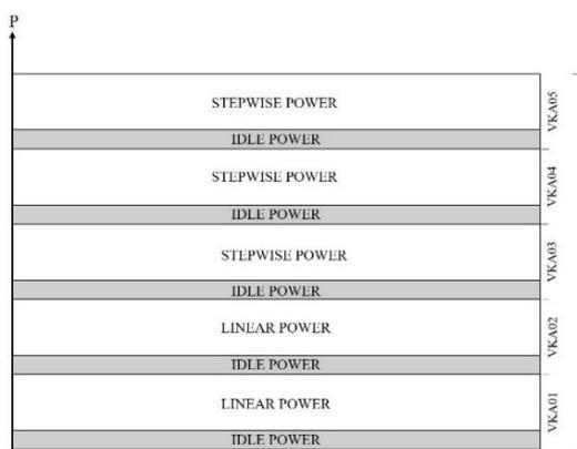
Figure 43: Sequential power of active chillers.
